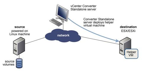
2 The helper virtual machine powers on, boots from the Linux image, connects to the source machine through SSH, and starts retrieving the selected data from the source. While you set up the conversion task, you can select which source volumes to be copied to the destination machine.
